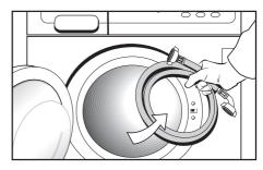
Connect the bent end of the hose to the threaded inlet of the electrovalve located at the rear of the washing machine
